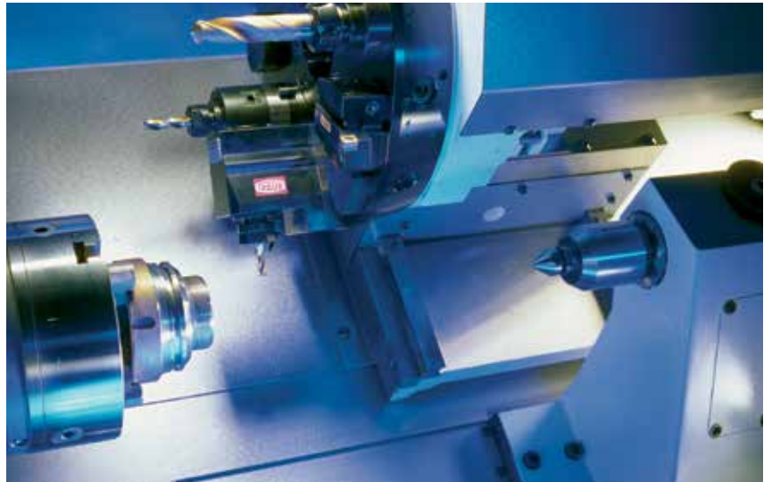
A generously dimensioned tooling zone and a fast indexing disc-type turret with 12 tool mounting bores. Internal coolant supply and directional logic indexing system are natural.
