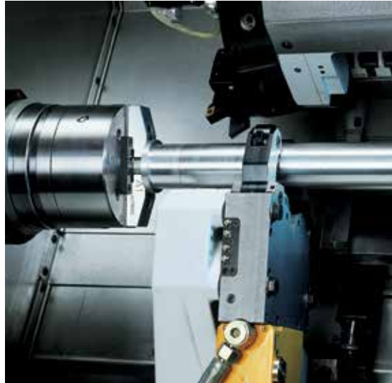
The universality counts with shaft-, preformed blanks- machining or bar work. Picture: Stationary steady rest.
