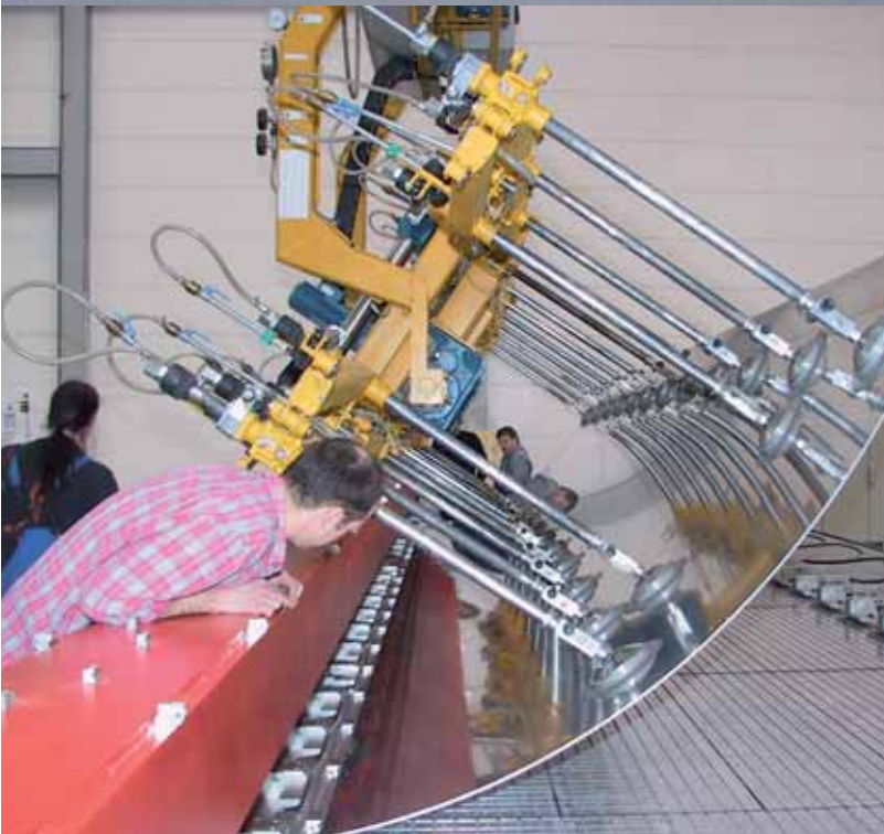
Clamping fixture for machining cylindrical pre-formed aircraft fuselage parts (13m x 4,10m) Parts are pressed down, rolled flat and clamped using vacuum as well as pneumatic and hydraulic clamps
