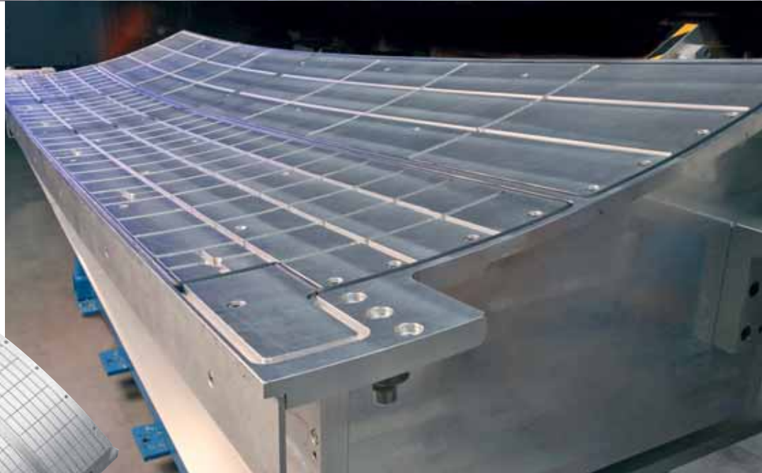
Vacuum fixture for clamping aircraft wing parts during friction-stir welding
