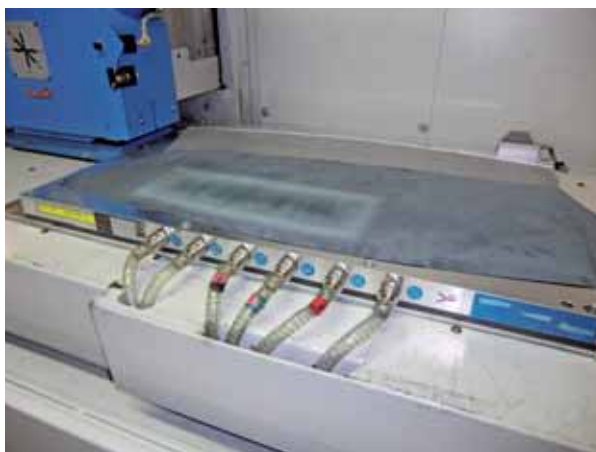
Application in automotive industry, leather clamped on visible side for grinding predetermined breaking points in areas of airbags on reverse side
