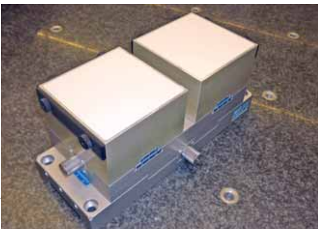
Double chuck system with two clamping surfaces which can be very accurately aligned to one another
