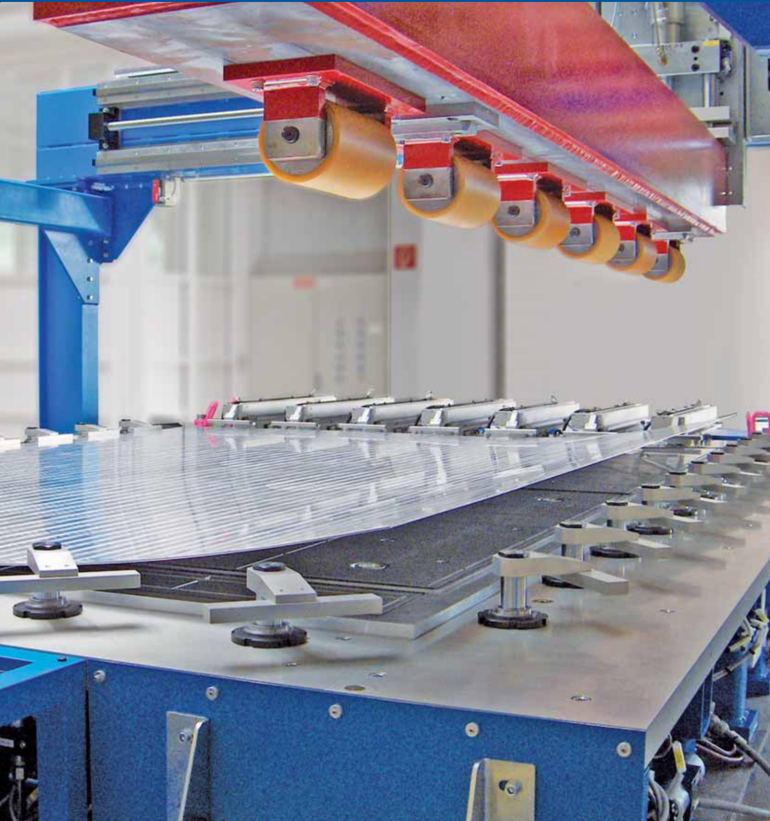
Roller bar vacuum system for precision machining pre-formed aluminium sheets
