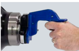
Insert & Unlock DC Collet
